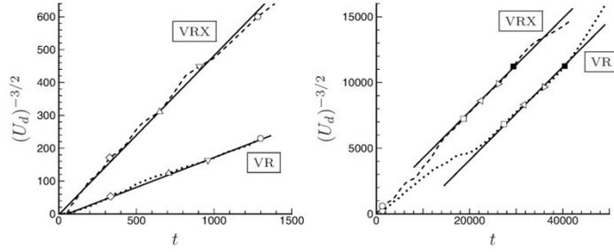
Figure 2: Similarity diagnostics for time-developing axisymmetric wakes:  $\cdots$ , Case VR;  $---$ , Case VRX. Variables normalised by initial maximum wake defect  $U_d$  and initial integral wake-width scale  $\rho_* = [(\ln 2/\pi)(I_d/U_d)]^{1/2}$  where  $I_d = 2\pi \int_0^\infty (U_\infty - U)r dr$ .
