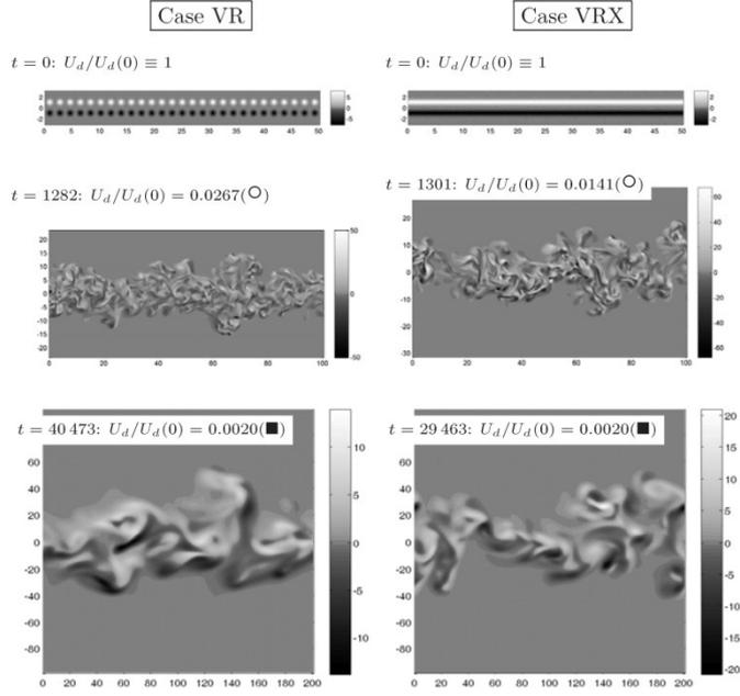
Figure 1: Evolution of vorticity contours for Cases VR and VRX.
