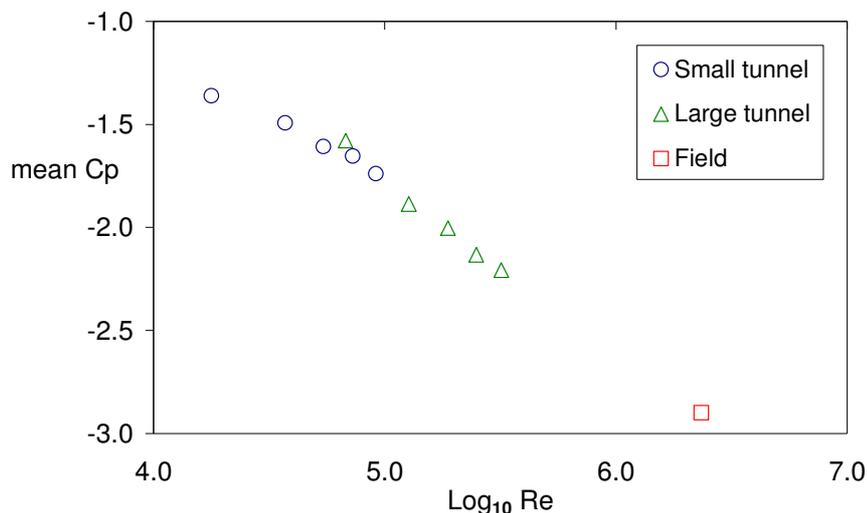
Figure 1 Mean surface static pressure under the vortex generated from the leading edge of a cube set at 45 degrees to the mean flow (position  $0.069 h$  from leading edge,  $0.356 h$  from side)
