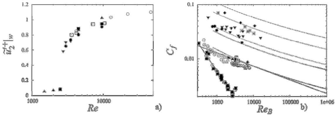
Figure 1: a)  $\tilde{u}_2^+|_w$  versus Reynolds number, for different rough surfaces. b)  $C_f$  versus  $Re_B$ . Solid symbols give the  $C_f$  of different surfaces from DNS the lines are obtained with different values of  $\tilde{u}_2^+|_w/u_B$  starting with  $\tilde{u}_2^+|_w/u_B = 0$  and with a 0.06 increment; the two dotted lines are at  $\tilde{u}_2^+|_w/u_B = 0.06$ , the thin with  $U_w = 0$ , the thick one with  $U_w = 0.2$ .
