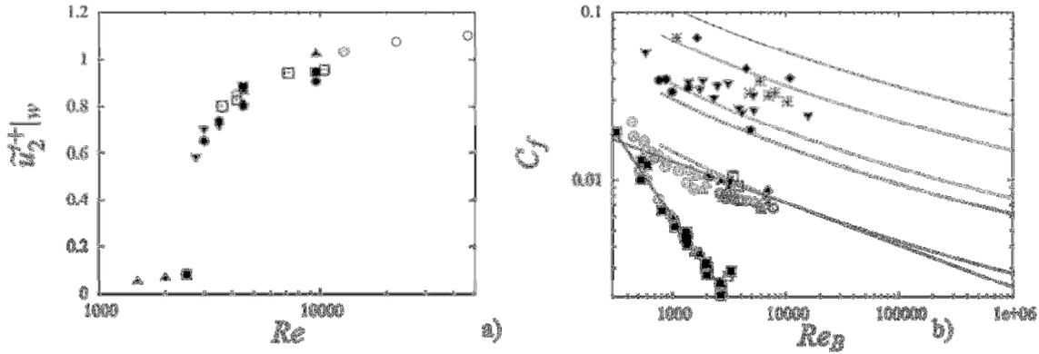
Figure 1: a)  $\tilde{u}_2^+|_w$  versus Reynolds number, for different rough surfaces. b)  $C_f$  versus  $Re_B$ . Solid symbols give the  $C_f$  of different surfaces from DNS the lines are obtained with different values of  $\tilde{u}_2^+|_w/u_B$  starting with  $\tilde{u}_2^+|_w/u_B = 0$  and with a 0.06 increment; the two dotted lines are at  $\tilde{u}_2^+|_w/u_B = 0.06$ , the thin with  $U_w = 0$ , the thick one with  $U_w = 0.2$ .
